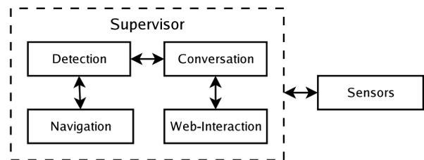
Fig. 8. Scheme of the application that integrates people detection with the other modules. Each block is a thread, all controlled by the supervisor.
