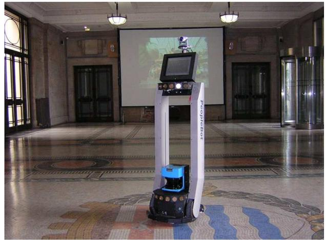
Fig. 7. ATLAS, the interactive museum guide robot. The test environment, in this case a wide foyer, has artificial lights, large door-windows and big movie-screens.
