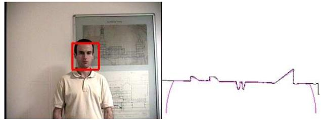
Fig. 10. Person too close to the wall. The legs pattern searched with a laser scan, on the right, can be confused with other objects in the environment. The face detector helps to resolve the confusion.
