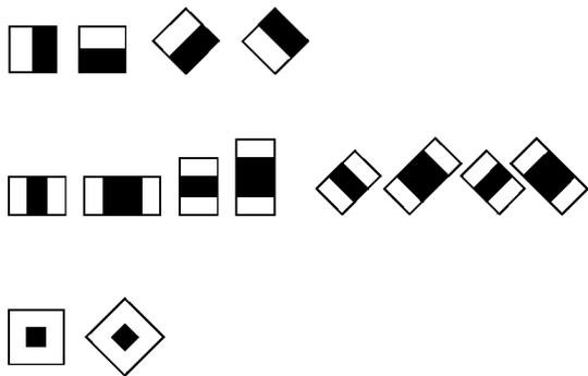
Fig. 3. Set of Haar-like features for face detection. The total amount of features contained in a  $24 \times 24$  window is about 120000.
