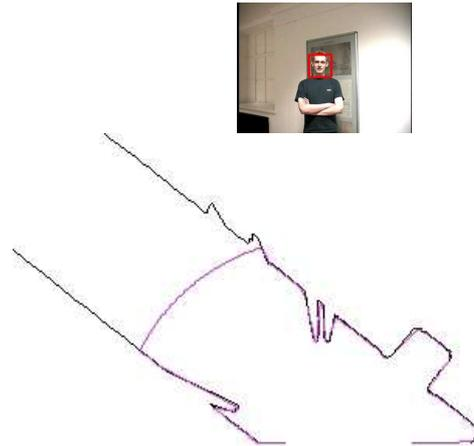
Fig. 1. Laser scan. The black line is the original laser output, the purple line is the output after filtering. In the middle we can notice the legs of a person (picture above).
