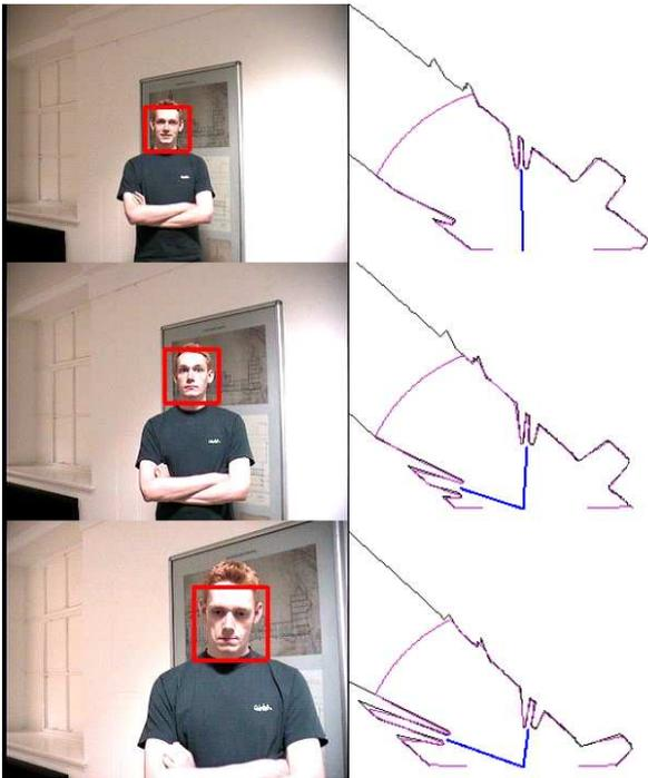
Fig. 9. Approaching a human. In the sequence we can see the detected face on the left and the relative laser legs detection on the right. ATLAS stops in front of the human (last snapshot) to start the interaction.
