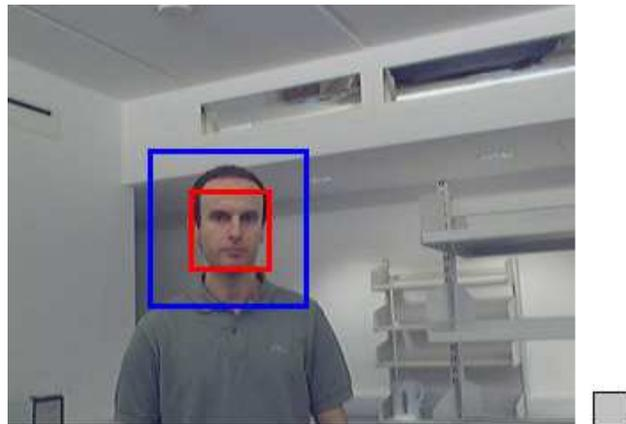
Fig. 4. At time  $t = 0$ , the whole image  $320 \times 240$  is scanned, with a minimum face size of  $20 \times 20$  pixel (small gray square on the right). The bounding box of the detected face (red square) is  $45 \times 45$ .
