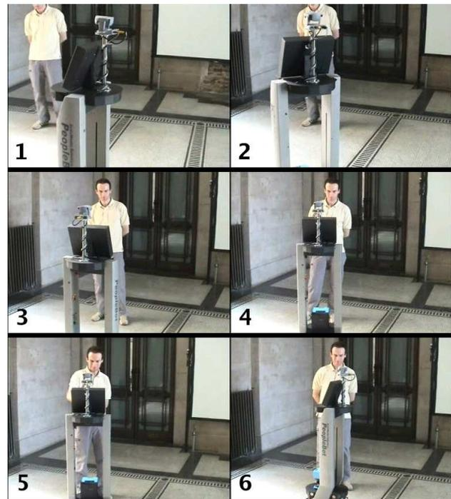
Fig. 13. Approach and interaction. In the sequence, ATLAS detects the person and approaches him (frame 1-3). After that, they interact using speech and the touch-screen (frame 4-5). Finally, when the interaction terminates, ATLAS turns and moves away (frame 6).
