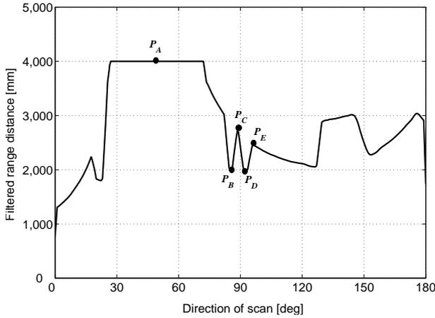
Fig. 2. Typical legs' pattern, identified by the sequence of points  $P_A \rightarrow P_B \rightarrow P_C \rightarrow P_D \rightarrow P_E$ .
