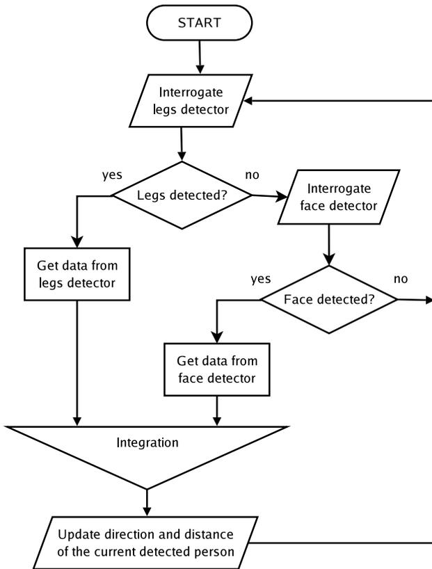
Fig. 6. Flowchart of the detection program. The information from the laser legs detector, more reliable, has the priority on the face detector.
