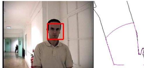
Fig. 11. Legs too close to each other. Instead of two columns, the laser shows just one big column. Even in this case, the face detector helps to resolve the ambiguity.
