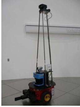
Fig. 3. Robot equipped with a SICK laser and a PTZ camera for the experiments. The camera used is the black one on the top.
