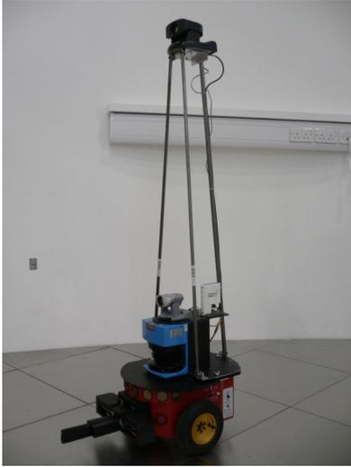
Fig. 5. Robot equipped with SICK laser and PTZ camera. The camera used is the black one on the top.
