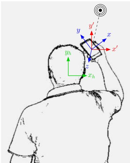
Fig. 4. Smartphone’s frame of reference  $\langle x, y, z \rangle$ ; 3D sound frame of reference  $\langle x', y', z \rangle$ ; and head frame of reference  $\langle x_h, y_h \rangle$ , with  $x_h$  oriented from the left to the right ear. The concentric circles on the top-right indicate the sound source (i.e. visual target).
