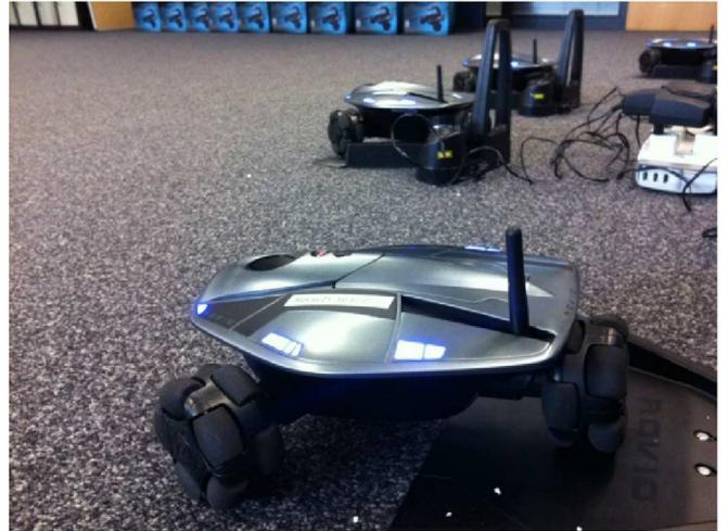
Fig. 2. Rovio, the mobile robot used for practical sessions.
